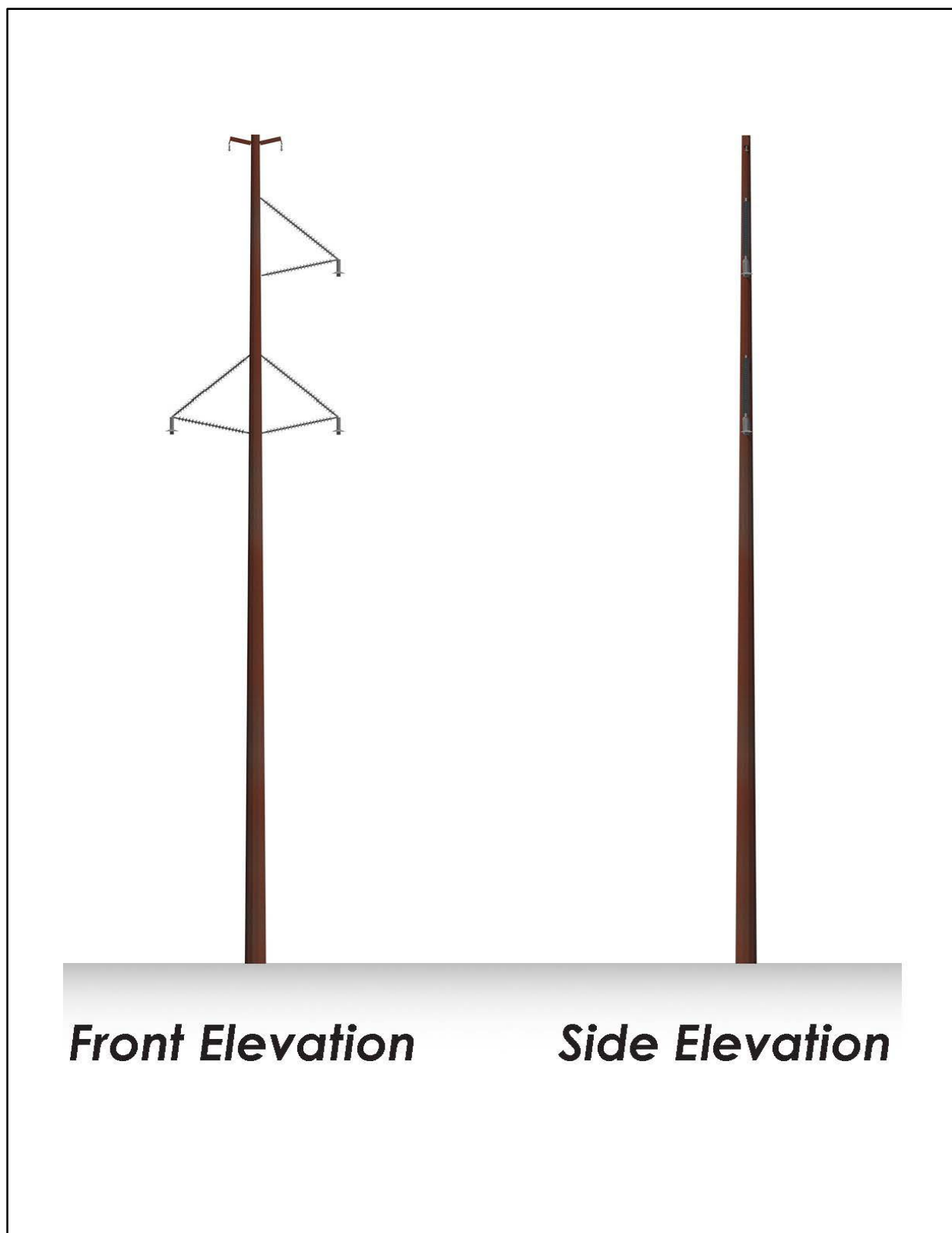
Exhibit G-1. Typical 230-kV tangent monopole structure.
